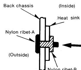
To remove a heat sink from the back chassis, first press nylon rivet-A from the inside in the direction indicated by the arrow as shown above, and extract the rivet to the outside. Next remove nylon rivet-B from the inside. Consequently, the heat sink can be removed from the back chassis.
